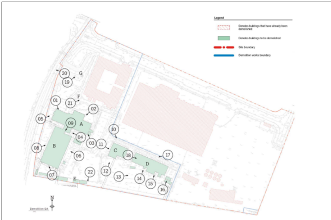
Green buildings are proposed to be demolished. Those highlighted in red are buildings which have already been demolished.
